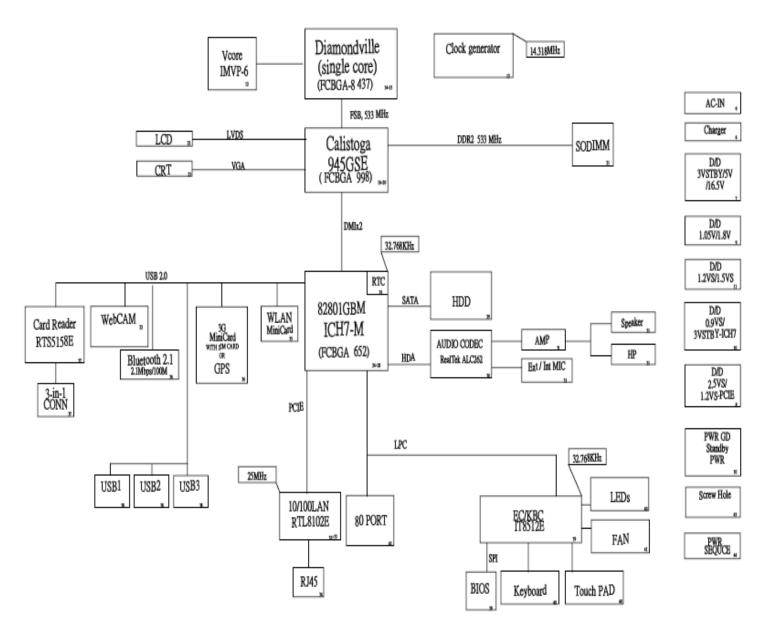
Figure 1-2 Computer Block Diagram
